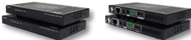
HD-H704K-SP HDBaseT 70m extender set - Compressed 4K-60 4:4:4, IR & RS- 232 18v PoE.
