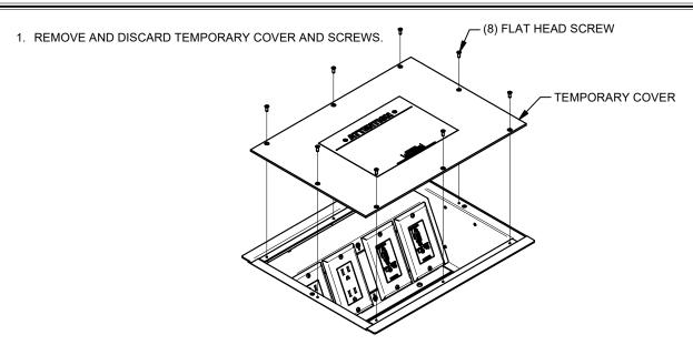
2. INSTALL ELECTRICAL DEVICES AND CONNECTOR PLATES IF PREVIOUSLY NOT INSTALLED. CLEAN AREA IN AND AROUND ENTIRE TOP EDGE OF BOX AND APPLY 1/4" CONTINUOUS BEAD OF RTV SILICONE SEALANT.
