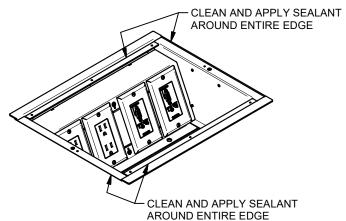
3. INSTALL COVER WITH SUPPLIED O-RINGS AND FLAT HEAD SCREWS. INSTALL FINISHED FLOORING MATERIAL.
