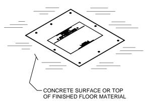
TYPICAL INSTALLATION HEIGHTS FLOOR BOX TEMPORARY COVER WILL EITHER BE INSTALLED DIRECTLY ON THE BOX OR SHIMMED BASED ON THE COVER AND FLOORING SPECIFICATIONS. SHIM KITS SOLD SEPARATELY (FL-500P-CSK).
