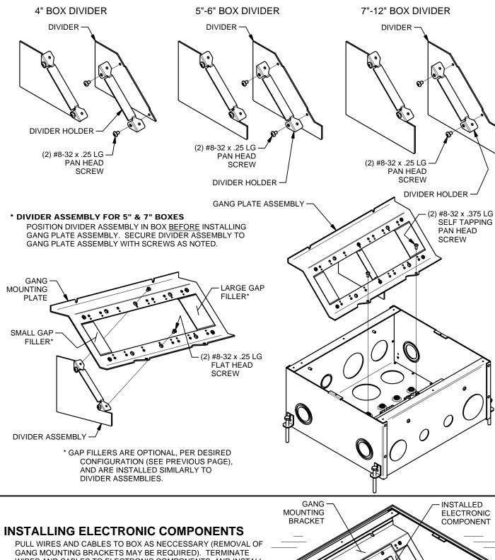
WIRES AND CABLES TO ELECTRONIC COMPONENTS. AND INSTALL ELECTRONIC COMPONENTS ONTO GANG MOUNTING BRACKETS. REINSTALL TEMPORARY COVER IF FINISHED COVER IS TO BE INSTALLED AT A LATER DATE.
