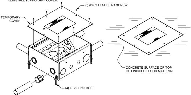
TYPICAL INSTALLATION HEIGHTS FLOOR BOX TEMPORARY COVER WILL EITHER BE INSTALLED DIRECTLY ON THE BOX OR SHIMMED BASED ON THE COVER AND FLOORING SPECIFICATIONS. SHIM KITS SOLD SEPARATELY (FL-600P-CSK). THE TEMPORARY COVER MAY NOT BE FLUSH WITH THE FINISH FLOOR IN ALL INSTALLATIONS.
