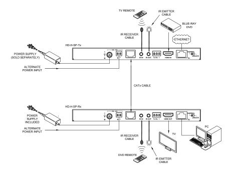
**NOTE:** It is only necessary to power one side (Tx or Rx)
