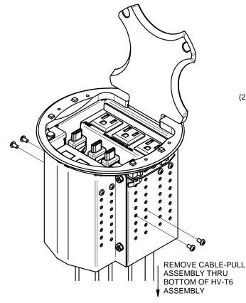
2. DETERMINE WHICH HDMI CABLE WILL BE REMOVED AND WHICH AUDIO HOLE WILL BE USED, AND DISASSEMBLE CABLE-PULL ASSEMBLY. RETAIN CABLE BUSHING AND DISCARD HOLE PLUG. ONE OR BOTH CABLE-PULL PANELS MAY NEED TO BE REMOVED.
