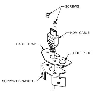
4. REINSTALL CABLE-PULL ASSEMBLY AT INDICATED HOLES.
