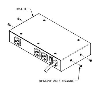
3. INSTALL HV-CTL TO BASE PLATE WITH SUPPLIED #6 HARDWARE.
