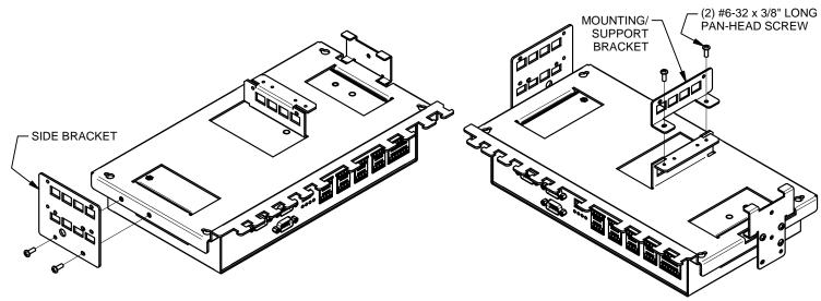
INSTALL DV-HSW4K-41 TO BASE PLATE WITH SUPPLIED M3 HARDWARE.
