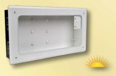
The PWB-353 Wall Box has an open face design with a white interior and white extended trim ring, including quick access to cables and connectors without cover removal. There are multiple knockouts for power, and openings for up to 6 single IPS connector plates. At 3" deep, it is designed for use in 3" or 4" stud walls. The extended trim ring provides a clean appearance while covering rough cuts in the drywall created during installation.
