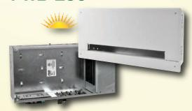
This unit is approximately 14.25"x7"x4" and has three single gang knockouts and one IPS knockout to mount up to six single IPS plates. In addition, a removable passthru enclosure provides an additional single gang knockout and can be used to isolate cables that the installer may need to pass through the backbox. The PWB-250-2KO is a version with 2" KO's available at the top and bottom of the box for special applications.
