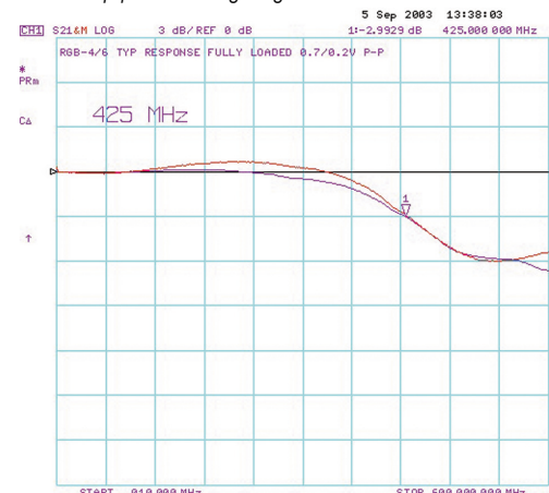
The above graph illustrates the typical frequency response of the RGB - 4/6. Notice that the curves represent a fully loaded unit and show the response to a 0.7V p-p and a 0.2V p-p input signals. It is important to observe that the overall flatness and upper limits are fairly independent of signal amplitude. This is an extremely important characteristic.
