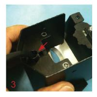
Replace Cable Cover by Slipping the Cable Cover Tab into the Milled Slot in the Top Cover. Replace 2 Screws from Step 1
