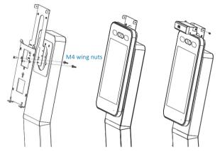
The figure below shows the process of installing the digital temperature measurement module on a standing pole when the module is to be used in combination with a face recognition terminal.
