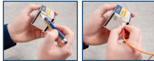
Figure 30 – "Wet to dry" cleaning methodology. Apply a small spot of solvent to the starting edge of a wipe. Holding the end-face connector perpendicularly, swipe the end-face from the wet spot to the dry zone.
