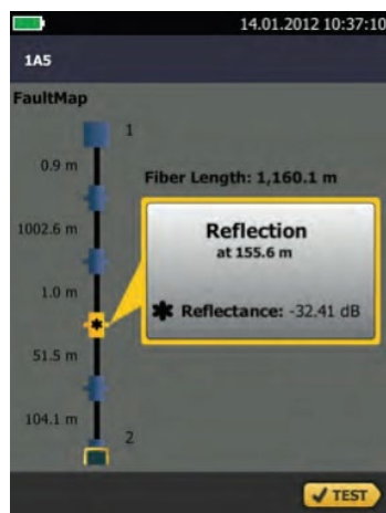
Figure 24 - FaultMap results view
