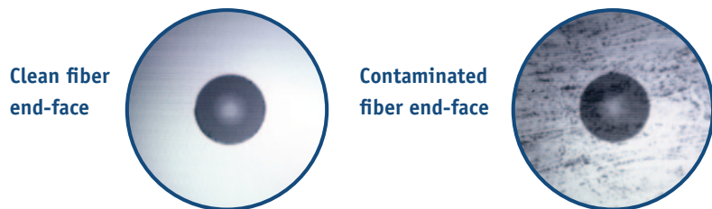
Figure 29 – Comparison between a clean and dirty fiber end-face
