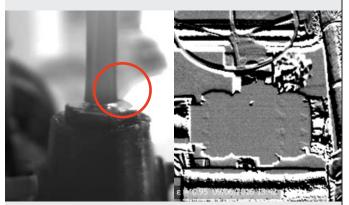
Thermal image of combined cycle unit shows a methane leak.
