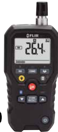
FLIR MR77 features a pinless moisture sensor and a wired pin probe.
