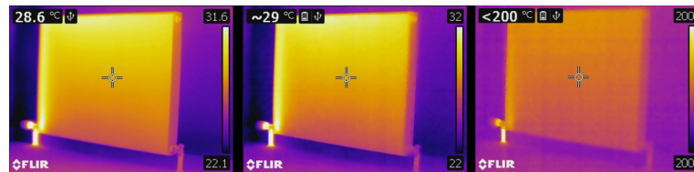
Figure 16.4 Images from a FLIR T440 with temperature ranges of -20 to +120^{\circ}\text{C} , (left, -4 to +248^{\circ}\text{F} ), 0 to +650^{\circ}\text{C} (middle, +32 to +1202^{\circ}\text{F} ) and +250 to +1200^{\circ}\text{C} (right, +482 to +2192^{\circ}\text{F} ). All other settings are unchanged.
