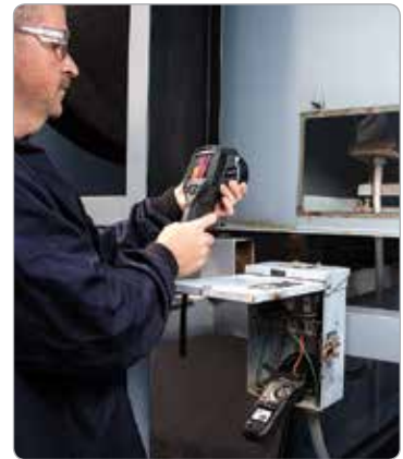
FLIR CM78 transmits real-time electrical measurements to FLIR IR cameras via METERLiNK
