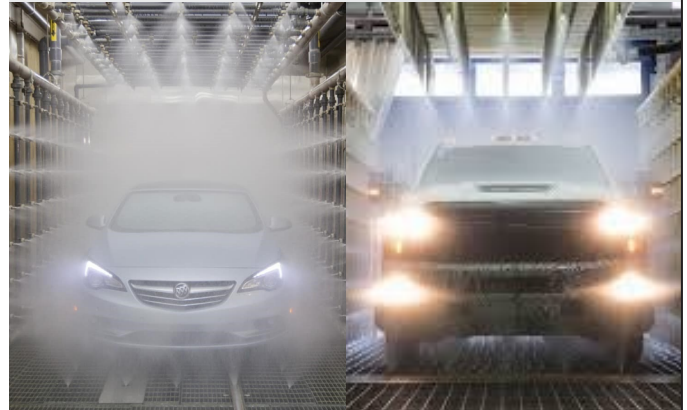
Water can penetrate even tiny gaps or seams in automotive weather seals, so it's important to find small leaks before they create bigger issues.
