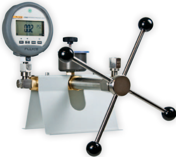
Combine the 2700G gauge with the P5510, P5513, P5514 (shown here) or P5515 Comparison Test Pumps for a complete bench top pressure calibration solution.
