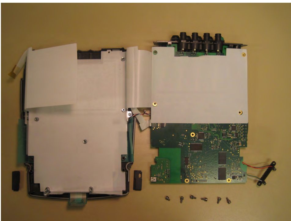
Fig. 6-3. Dismantling step 3 (PCA separated from chassis)
