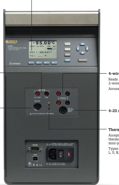
**4-wire PRT/RTD input** Reads a 4-wire, 3-wire, or 2-wire PRT/RTD Accuracy ±0.02 °C
