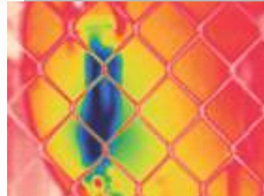
Passive autofocus systems may only capture the near-field subject (fence).
