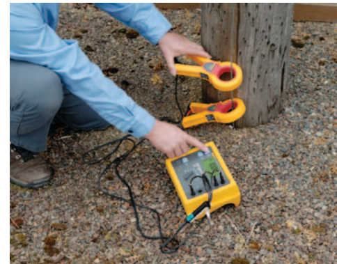
With the Fluke 1625 GEO Earth Ground Tester you can perform 3- and 4-pole earth ground measurement, 4-pole soil resistivity testing, 2-pole resistance measurement ac, 2- and 4-pole resistance measurement dc, selective testing, and stakeless testing.
