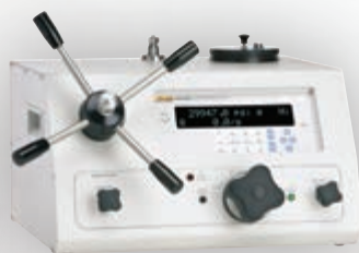
6531, 6532 Electronic Deadweight Tester See pg 30
