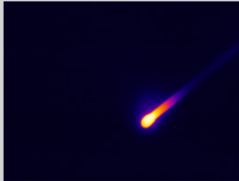
Figure 4. This image of a match right after it was extinguished was captured with a TiX560 camera and a standard lens.
