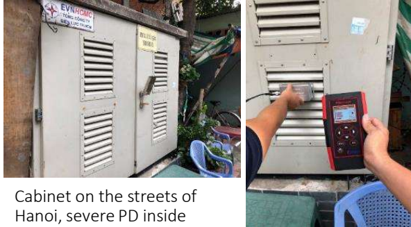
Routes across the city to inspect distribution lines, cabinets & transformers using ultrasound
