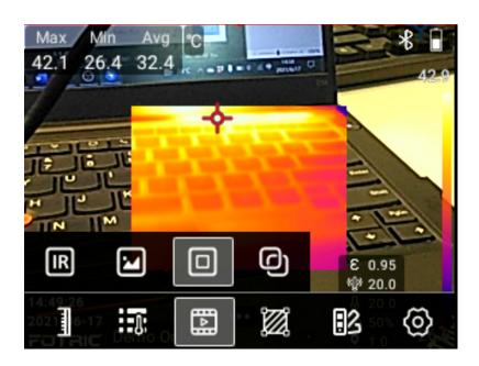
By default, the thermal display area is 1/4 of the entire screen. Users can adjust the thermal image areas and position by touch-screen, as the below following images:
