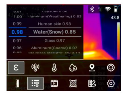
E The emissivity settings of the FOTRIC thermal imager have 2 options: Fullscreen emissivity correction and partial emissivity correction.
