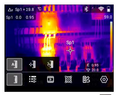
The thermal imager supports auto scale, auto scale, manual scale and touch scale modes.
