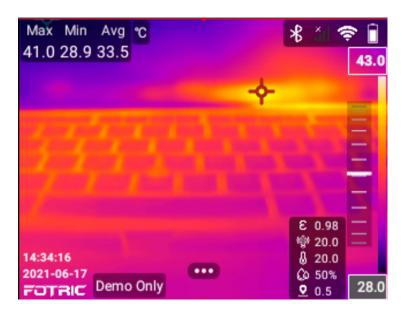
As shown in the figure below, the lower limit of the temperature scale can be adjusted separately by using the slider
