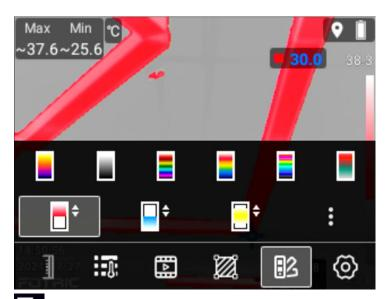
color alarm (isotherm): above temperature alarm, for quickly finding the high-temperature abnormal area of the target object.
