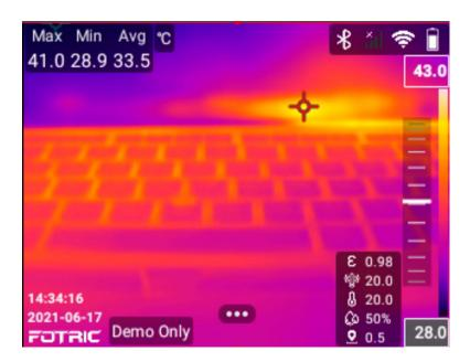
A short press on the direction key will increment the span by 0.1 degree. When held on, the increment will gradually increase
