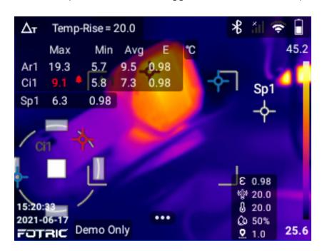
Lowest temperature: alarm will trigger for the minimum temperature of ROI;
