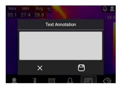
Text annotation can be added to the thermal image file by the virtual keyboard on the screen.
