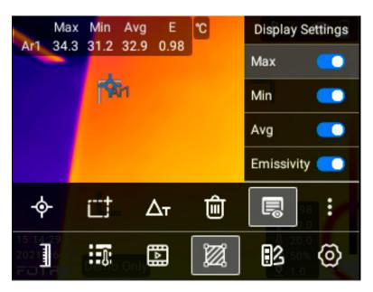
The available options for display are maximum, minimum, average temperature and emissivity. The default display is the maximum temperature.
