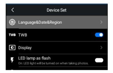
TWB mode: TWB is named Thermal White Balance. It balances color distribution on the entire temperature span of the image.
