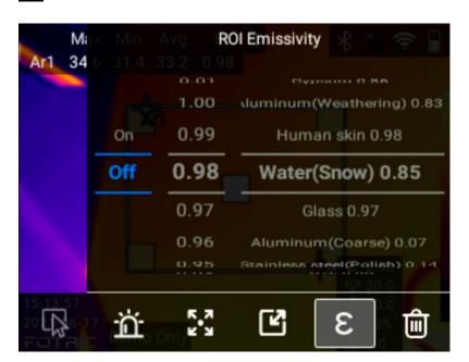
For the emissivity of material that is not included in the chart, you may find it in the emissivity table at the end of this manual. The 'Partial emissivity setting' feature is available through touch-screen and press-button. If you need to set specific emissivity for different ROIs, please follow the procedures as below:
