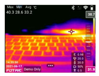
As shown in the figure below, both upper and lower limits of the temperature scale are locked and cannot be adjusted:
