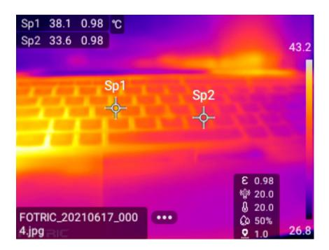
On the Image Freeze Interface, the image can be edited or analyzed before save. Press the capture button again to save the image.
