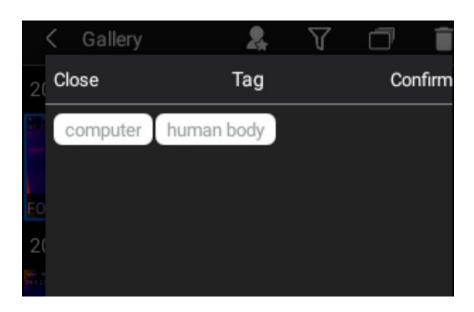
Click on the desired tag contents, then click 'confirm' to filter all the files that contain the tag. Click the icon again to undo the filtering. For more information, see section 6.4 of this manual
