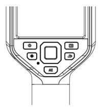
The AI programmable key can call upon different functions according to the user's need. It is available on the main interface, image freeze interface, and gallery's image analysis interface.
