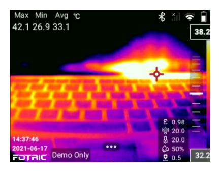
As shown in the image below, the upper and lower limits are selected. And the range of temperature scale can be adjusted by up and down direction key
