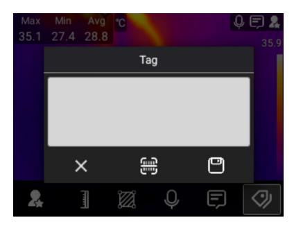
In the image freeze interface, Tag information can be inputted by QR code scanning and virtual keyboard
