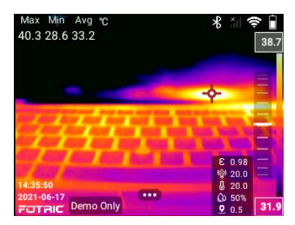
As shown in the image below, the lower limit is selected. And the lower limit of the temperature scale can be adjusted by up and down direction key
