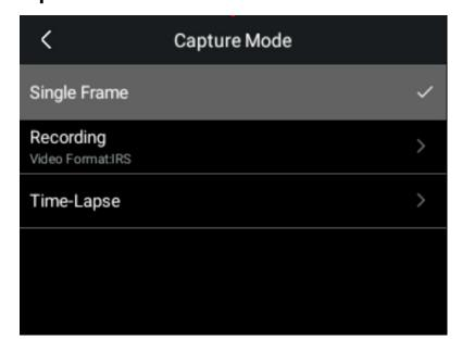
The device can be set to take single frame picture, record IRS radiometric /MP4 videos or time-lapse pictures.
