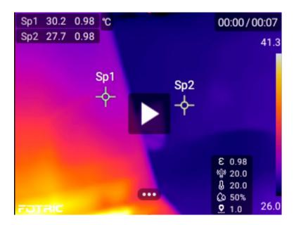
Users can preview the radiometric image before saving it. On the freeze interface, videos can be analyzed. Pressing the trigger button again to save the video.
