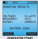
**GENERATOR START** Test the state of health of generator starting batteries.
