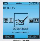
**QUICK TEST** Start a test on a single cell or monoblock without setting up
