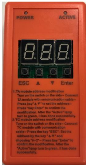
The default TC address is 241, but you can choose an address from 241 to 247. If you are monitoring only one battery string, the address can remain the default.
