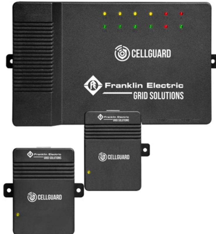
Franklin Electric Grid Solutions Wired Battery Monitoring System (BMS) consists of battery sensors (TA) that measure voltage, temperature, and the internal resistance of the battery. TC sensors measure the battery string current and ambient temperature. Both sensors report data to the Base Controller (BC) module:
