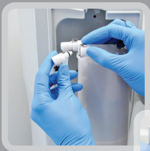
Quick-connect cartridge replacement
