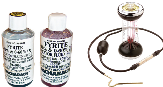
Figure 7. Chromous Chloride (Blue) and Potassium Hydroxide (Red) Reagent Fluids
