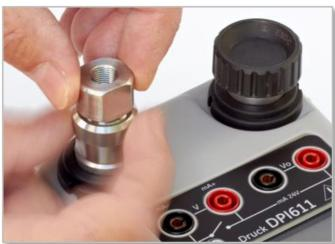
Making a leak-tight pressure connection in the field is inevitably frustrating. The DPI 611 comes with a quick-to-fit adaptor system
