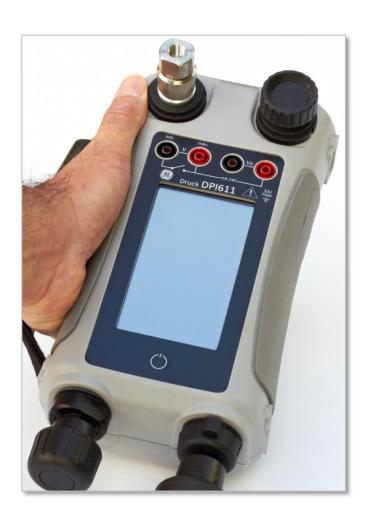
The DPI 611 is truly a hand-held pressure calibrator being 50% smaller and 33% lighter than the DPI 610
