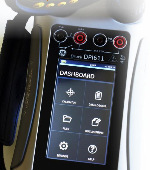
The DPI 611 is a simple to use "everyday" tool for maintaining and calibrating pressure instruments. It also has the advanced features of the DPI 620 Genii for automating calibration procedures, calculating errors and interfacing with calibration and maintenance systems.
