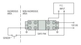
Programmable SAFE-PAK, P/N 54825, providing simple on-off functions for hazardous location, and interfacing with TTL or AC logic input of programmable controller. \*Temperature, pressure, position, flow or level.
