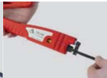
Press the clamp until the thimble is completely inserted in the connector and insert the crimped cable, and fasten it with the relevant cable holder.
