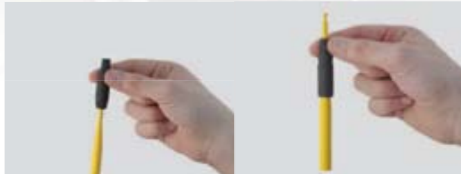
With the right hand, completely insert the MC3 connector into the thimble
