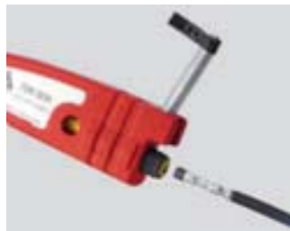
Press the clamp until the thimble is completely inserted in the connector and insert the crimped cable, and fasten it with the relevant cable holder.
