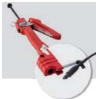
Insert the thimble with the connector into the appropriate housing for the cable
