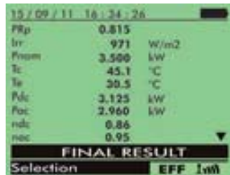
Testing result of photovoltaic system
