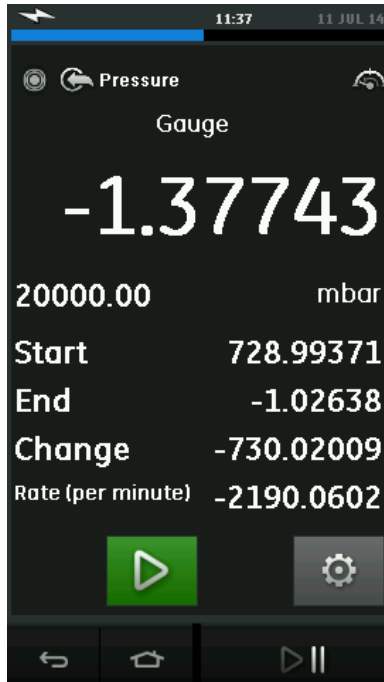
Figure 2-27 Leak Test Example
