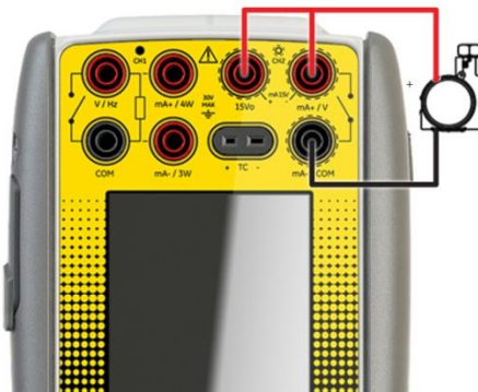
Figure 8-3 Example Connection Diagram FOUNDATION™ Fieldbus – Internal Network
