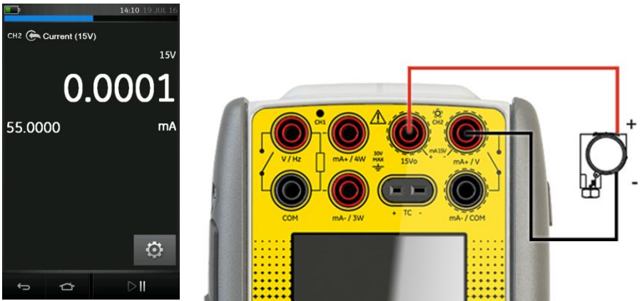
Figure 2-16 Measure Current on CH2 with Internal 15V Loop Power, Range \pm 55\text{ mA}
