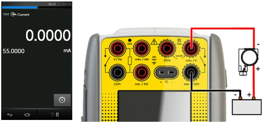
Figure 2-14 Measure Current on CH2, Range \pm 55 mA
