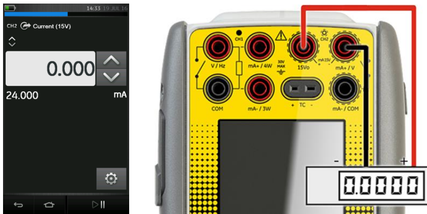
Figure 2-17 Source Current on CH2 with Internal 15V Loop Power, Range 0 to 24 mA
