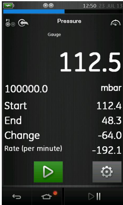
Figure 3-10 Leak Test Example
