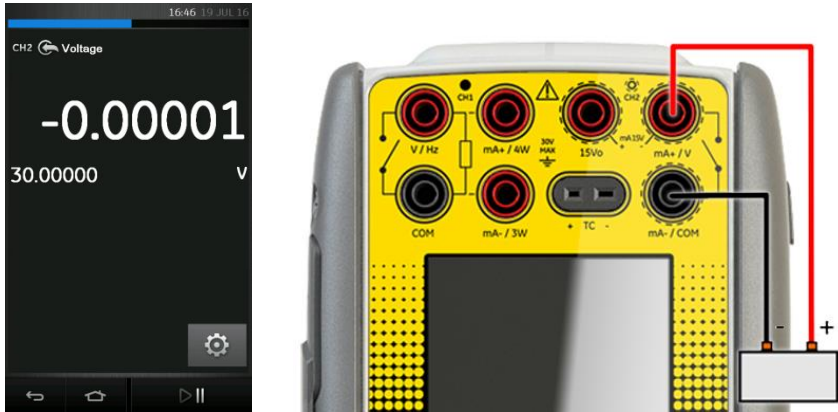
Figure 2-19 Measure DC Volts or DC mV on CH2, Range \pm 30 V
