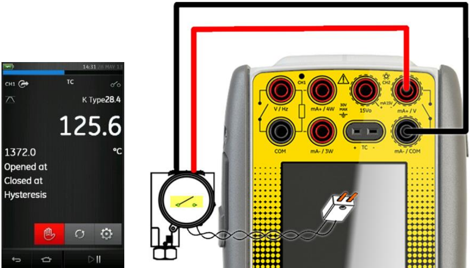
Figure 2-29 CH1 Thermocouple Source, CH2 Switch Test
