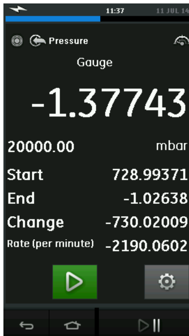
Figure 2-25 Leak Test Example
