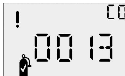
Spanning Failed Screen
