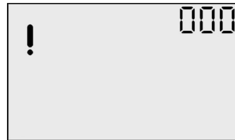
Sensor Missing Error Screen
