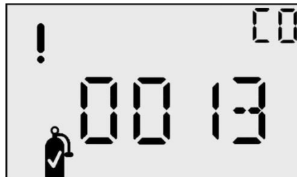
Cal Failed (!) Screen
