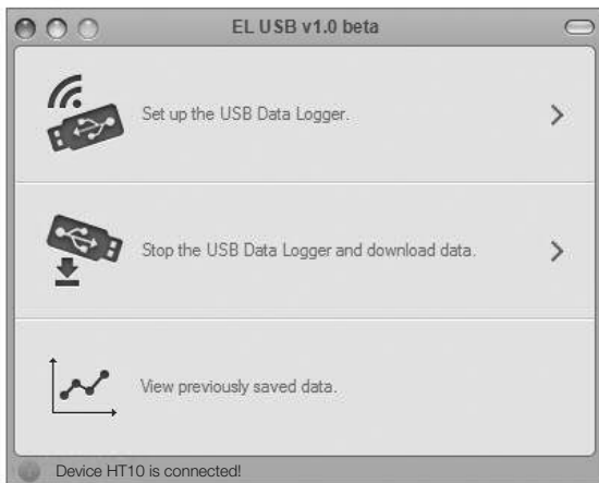
Fig. 2. The three options made available by plugging the HT10 into a USB port
