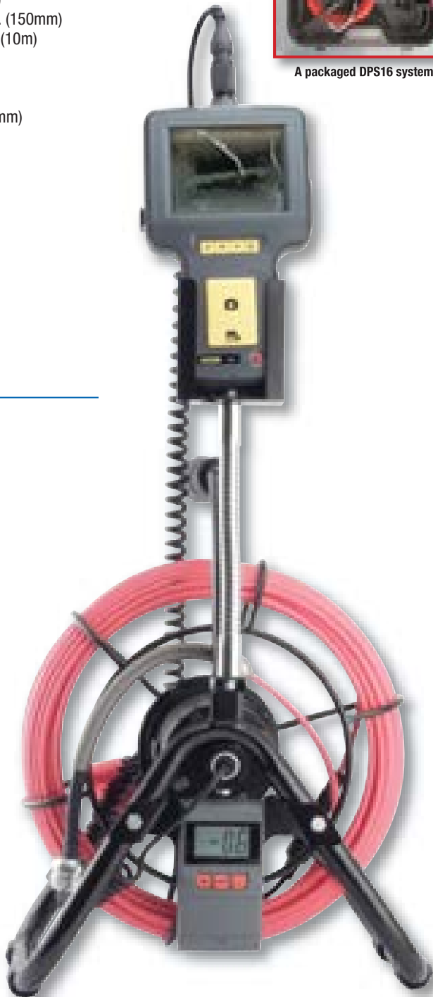
The DPS16/P16PIP probe is flexible enough to make two 90° bends in a 1.6 in. (40mm) diameter pipe
