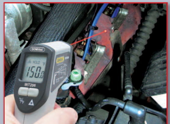
With a 600^{\circ}\text{F} measurement ceiling, the unit can handle any automotive application
