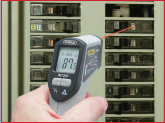
The IRT206 makes it easy to detect overheated circuits
