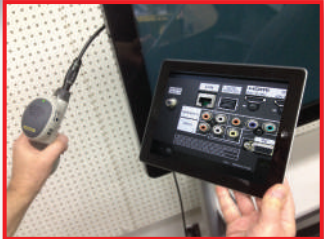
iBorescope makes it easy to identify the jacks on the back of rack or wall-mounted equipment
