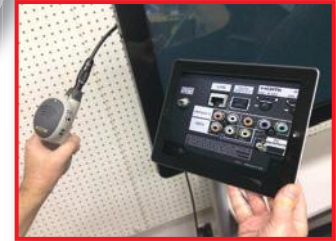
iBorescope makes it easy to identify the jacks on the back of rack or wall-mounted equipment
