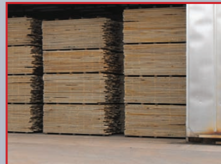
A kiln will dry these hardwood boards to a moisture content of <10%
