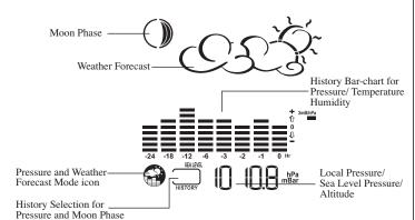
NOTE: An altitude display of 99o, is actually 990 feet, etc. Pressure can be displayed as: "inHG" (default) inches of mercury, "mmHG" is millimeters of Mercury and "hPa/mBar" is scientific hectoPascal.
