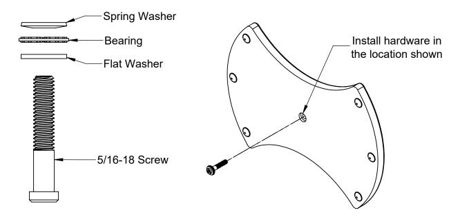
**Step 3:** Add the remaining hardware to the top of the Base as shown.
