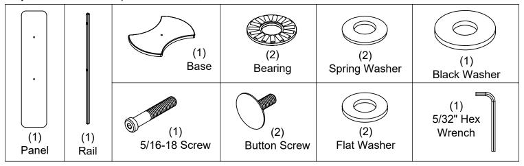
**Step 2:** Assemble the Base as shown using the 5/16-18 Screw with a Flat Washer, then a Bearing, and finally a Spring Washer. Please note the Spring Washer should have the cone pointed towards the Bearing.
