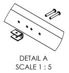
**Step 4:** Using a table (6) feet or more in length, organize the legs and cross brace as shown below, hand tighten 10-24 x 1" screws with acorn nuts.
