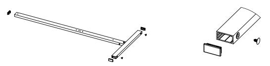
Step 3: Install bracket onto legs using 10-32 x 1-1/4" screws, thread screws into bracket. Do not tighten.
