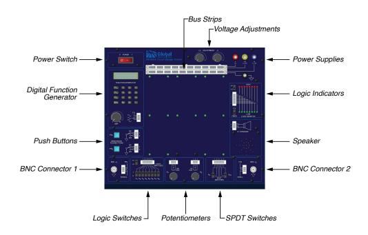
Figure 1 PB-503A Components
