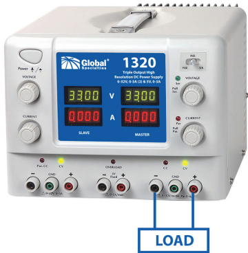
Figure 6. Parallel Tracking Mode
