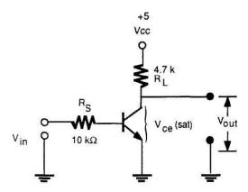
The circuit is operated in the saturated region. When the input is Vcc, the circuit is saturated if Ic » (beta) X Ib. The output is a low voltage (0.2-0.6 V for a silicon BJT). When the input is near ground, the transistor is cut off and the output is Vcc.
