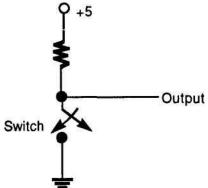
The contacts of the mechanical switch will bounce between states when the switch is activated. This can cause false triggering in logic circuits connected to the switch.
